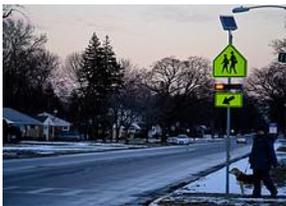
*Pedestrian flashing lights at both sides of this crosswalk*
